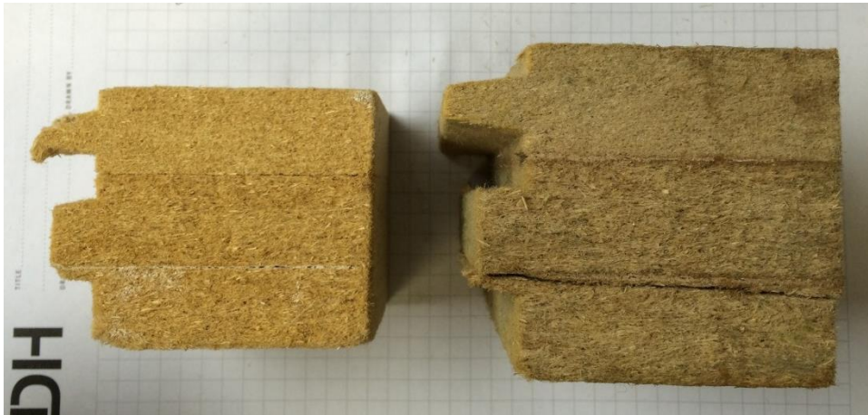
Agepan insulation before & after 60 days, 100% RH
